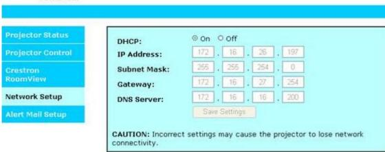
**DHCP**: The DHCP server of the domain will assign an IP address to the projector automatically
